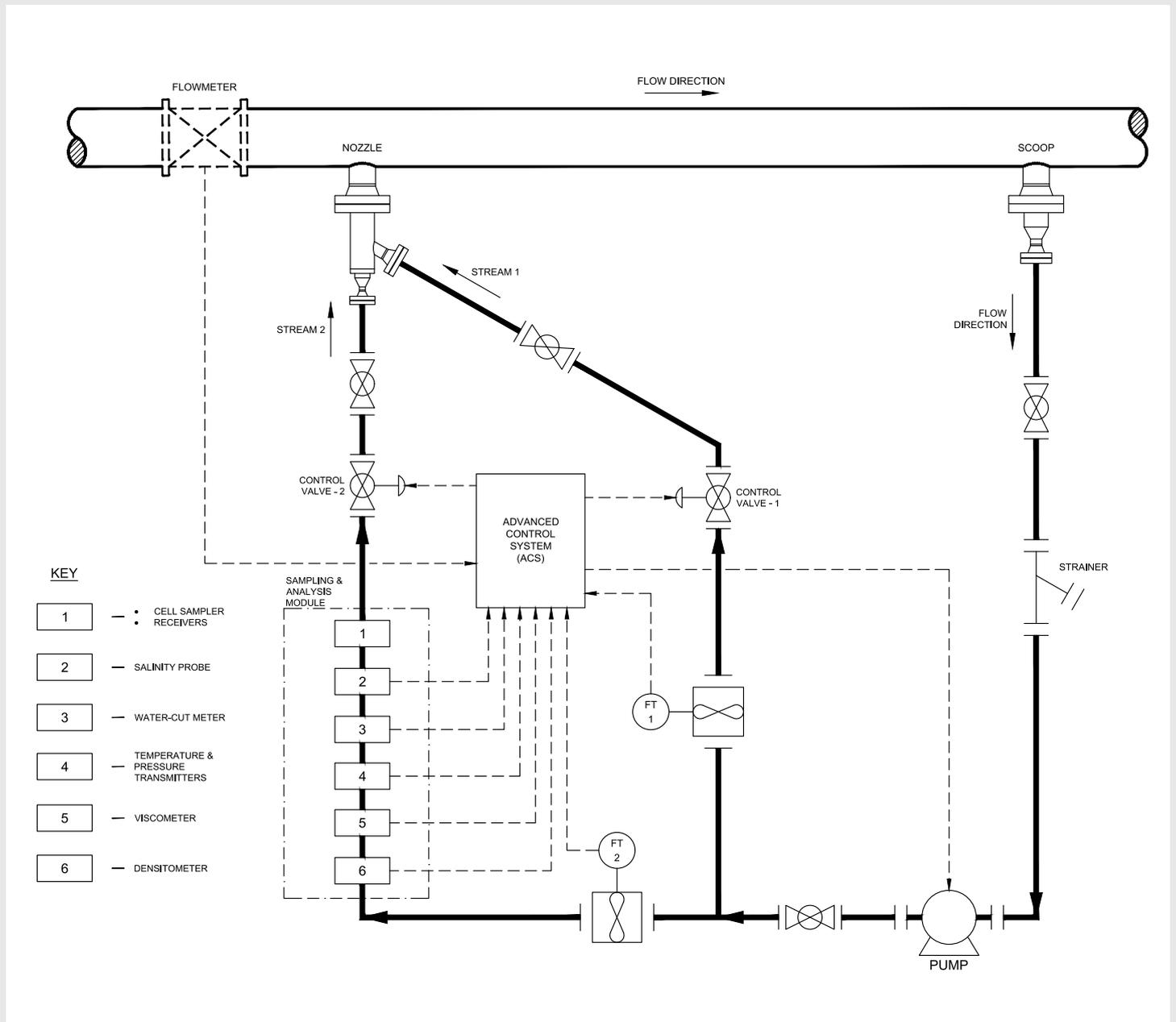
Figure 3 - Typical SmartMix® System Configuration
