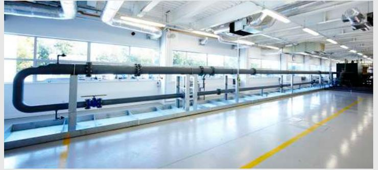
Figure 5 - OGM's Oil-Water Multiphase Loop (10") used to conduct validation and proving tests for SmartMix® Technology
